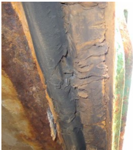
Figure 5: Hardened indented rubber seals
