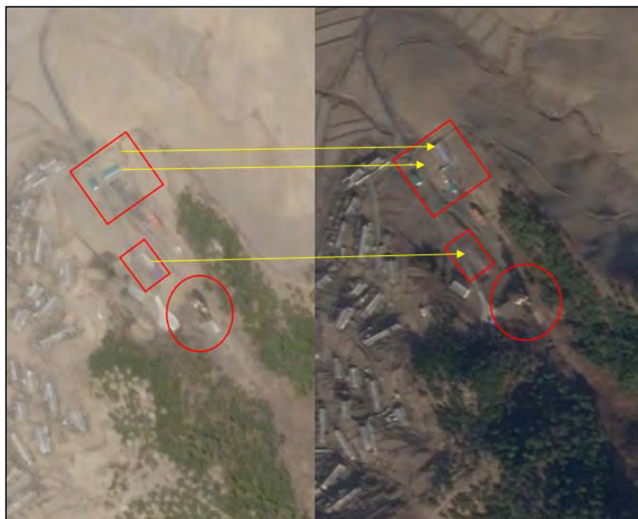
Figure 63.2: Developments at the vertical engine test stand infrastructures between 15 April (left) and 2 December 2019 (right): destruction of two buildings, construction of three buildings (see series of pictures below). The test stand is in the centre of the red circle.
