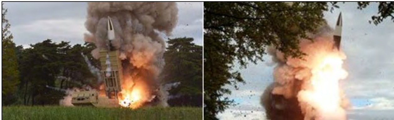
Figure 58.4.2: The two SRBMs launched on 16 August 2019 resemble the US MGM-140 ATACMS and the TEL chassis built on the DPRK Pokpung-ho battle tank chassis derived from T62 and T72 (see Figure 53.3.2)
