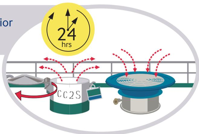
Check tank atmosphere for oxygen content and toxic gas
