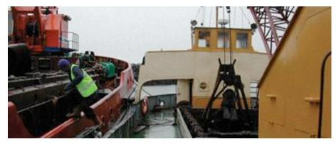
Figure 9: A crew member leaping from one vessel to another as no correct means of access is rigged
