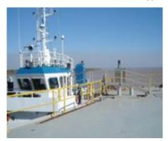
Figure 11: Correctly rigged gangway between double banked vessels
