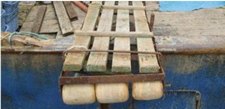
Figures 2 and 3: Means of access incorrectly rigged
