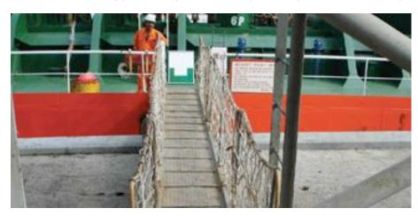
Figure 4: A correctly rigged gangway
