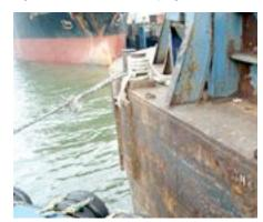
Figure 10: Incorrect access between two vessels
