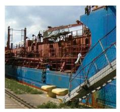
Figure 7: A gangway rigged taking into account the shore side hazards e.g. mooring bollards and crane track
