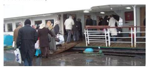
Figure 14: The area between the gangway and vessel's railing left unguarded
