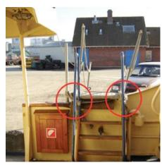
Figure 5: Gangway incorrectly secured to the vessel
