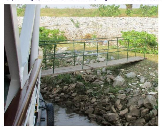
Example B: Gangway has not been manufactured by recognised international standards, is not properly secured and the slope is > 30 degrees.
