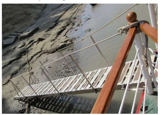
Example C: Gangway has not been manufactured by recognised international standards, is not properly secured, has no side screens or handrails provided and is not well lit.
