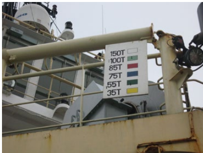
Figures 20 and 21 SWL system for shackles utilising colour coding
