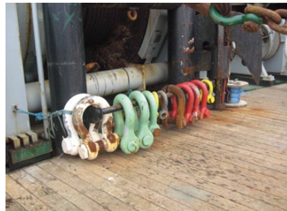
Figures 20 and 21 SWL system for shackles utilising colour coding
