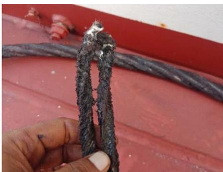
*The effect of poor lubrication*
