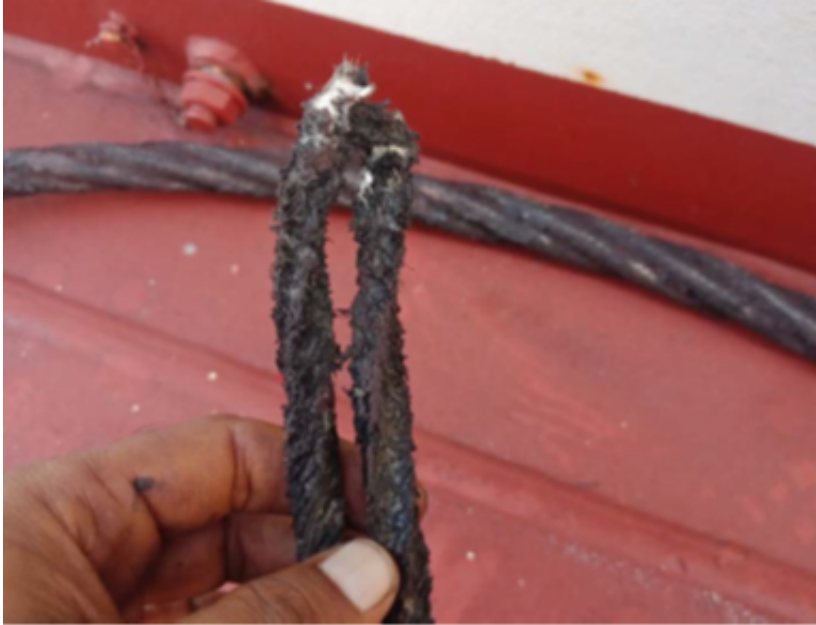
The effect of poor lubrication
