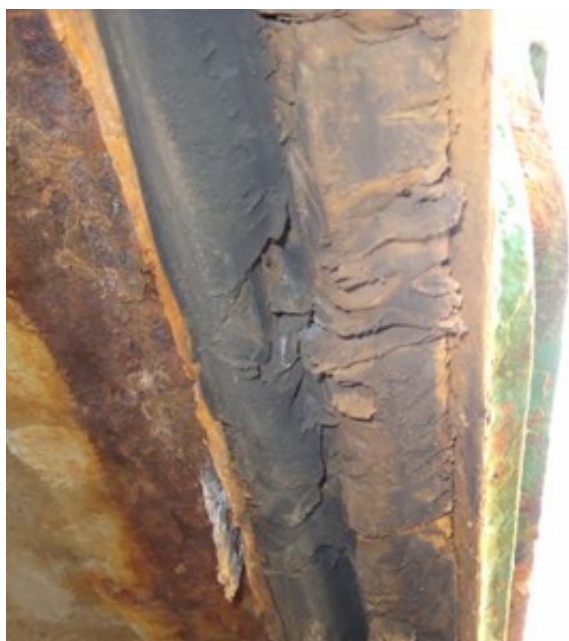
Figure 5: Hardened indented rubber seals
