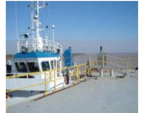
Figure 11: Correctly rigged gangway between double banked vessels
