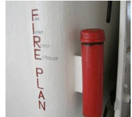
Figure 6: A typical fire plan located in the vicinity of the vessel's access
