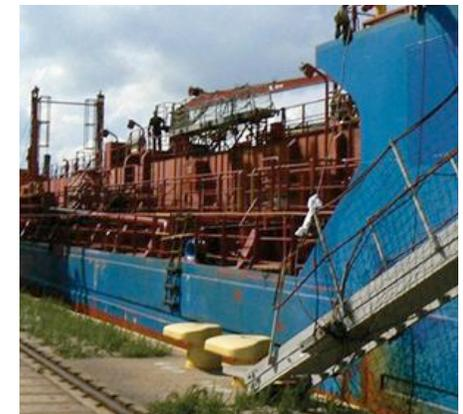
Figure 7: A gangway rigged taking into account the shore side hazards e.g. mooring bollards and crane track
