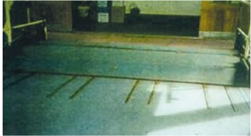
Shortly after passengers started to board, another vessel berthed in an adjacent wharf creating some wake. The combination of the wake and wave actions in the harbour caused the ferry to surge and roll. The movement resulted in the hydraulic ramp fitted to the ferry rising a few inches above the connecting hydraulic ramp fitted to the jetty. When the vessel rolled back a passenger's foot was trapped between the ramps.
