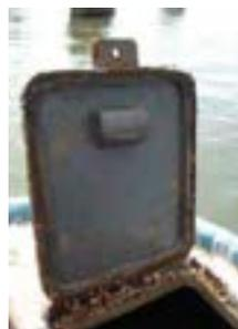
Figure 9: Hatch without a locking pin
