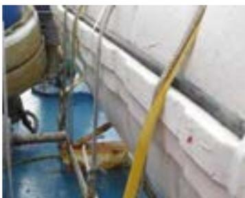
Figure 10: Incorrectly stowed life raft
