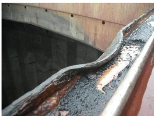
Figure 2: Damaged cargo hatch sill
